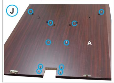
**STEP 11:** Use **Screws (I)** to secure **Brackets (P)** to the bottom of one of the **Table tops (A)** nearest the outside of the **Sash Locks (Q)**, Making sure they hang half-way over the edge.
