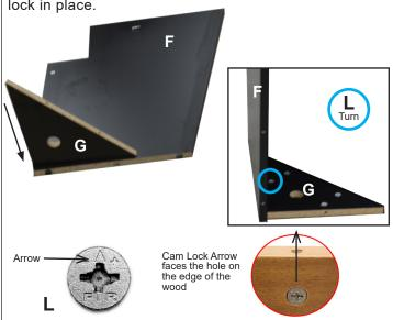
STEP 5: Connect the Front Leg Panel (D) to the Pivoting Cam Pin (K) on the Right Leg Panel (F) and Cam Pin (J) to the hole on the Support Block (G).
